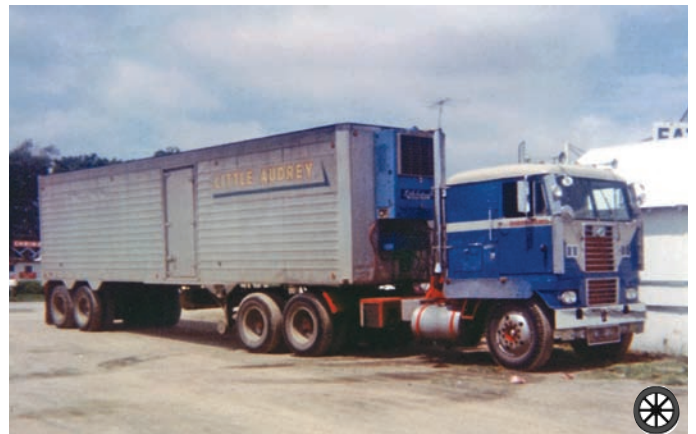
Below: This decked-out 931C Diamond T even had large mud guards on the cab sides. I think the red unit box on the frame was an early design of an APU. The rig had lots of mirrors. (Summer 1959)
