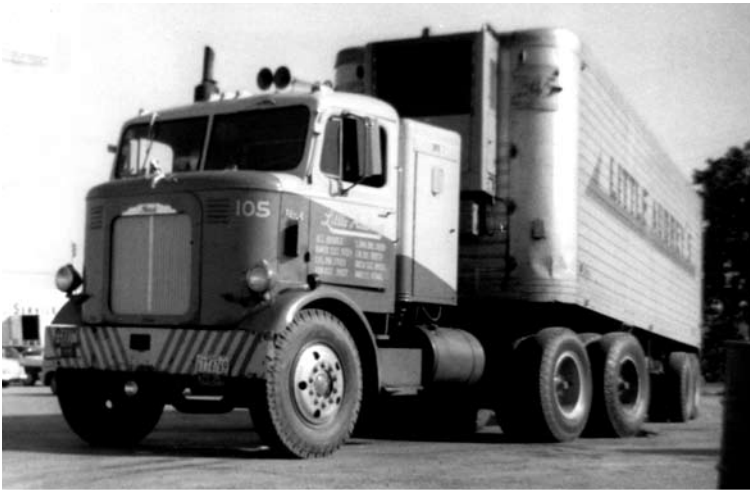
This red International RDC-405L had twin horns, spotlights, and very loud twin straight stacks. It was powered by a 220 Cummins with 10-speed Roadranger and was pulling a Brown trailer with blue Little Audrey signs. (August 1956)
