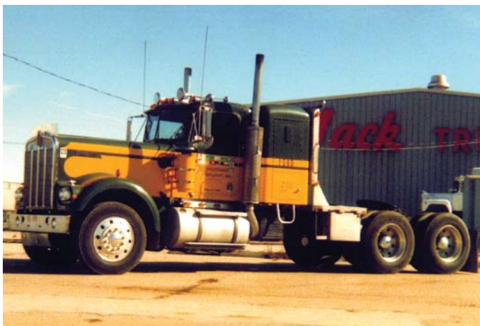
The standard Kenworth paint design, drom deck, and Cat power make this W900A extended hood tractor with 36-in sleeper a classic looking workhorse.
