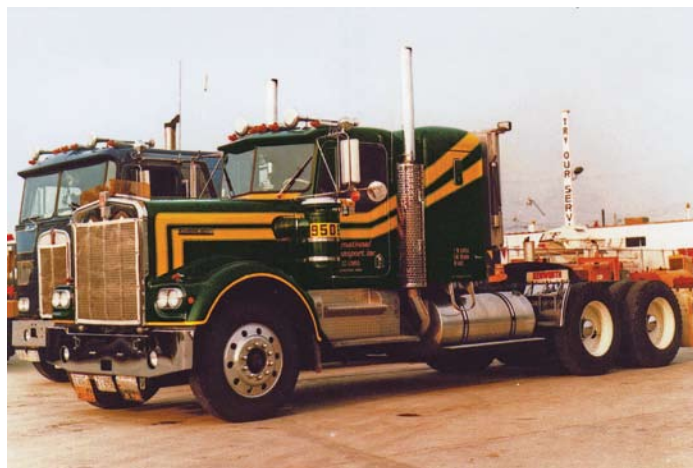
Another nice Kenworth W900A, tractor No. 9508 in the Heavy Haul Division has a short hood and 36-in sleeper.
