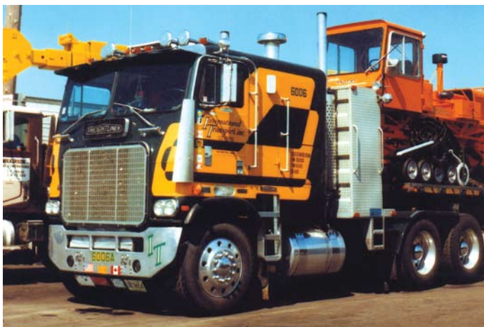
This Freightliner Powerliner double bunk tractor is a rare sight. Its eye-catching paint and custom Merritt headache rack really stand out. The Powerliner was designed to accommodate engines 400 hp and bigger, the biggest being Caterpillar 3408s, Cummins KTA 600s, and Detroit Diesel 8V92TAs. This was a Canadian Division tractor.
