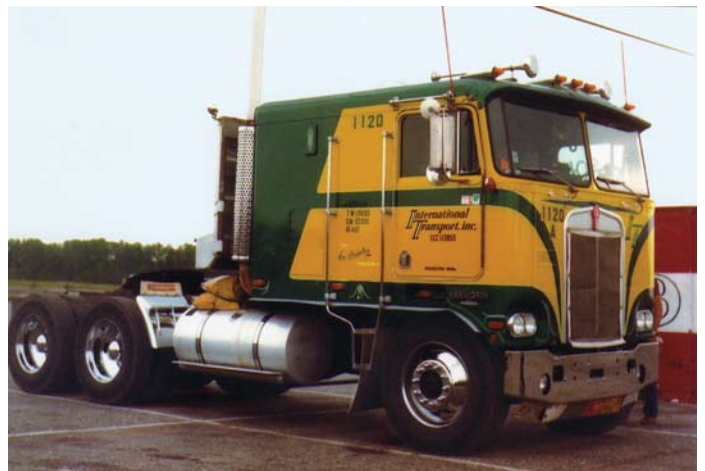
This sharp Kenworth K100 double bunk, tractor No. 1120, shows the owner's pride with its subtle pin striping and chrome steel wheels all around. The chrome steel Budd wheels always looked great on early model tractors.
