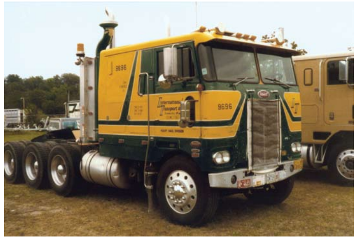
An early 1970s Peterbilt 352 double bunk tri-axle tractor, this unit in the Heavy Haul Division was also owned by Erv Fenske Jr.
