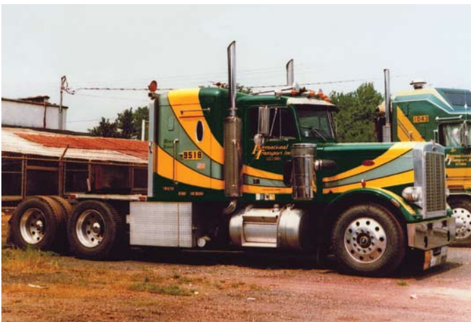
This nice Peterbilt 359 was not painted the standard IT green. The factory 36-in sleeper appears to have been made larger and taller. Other custom features include generator, windows on the sleeper, and a drom deck. It made a nice Heavy Haul Division combo.
