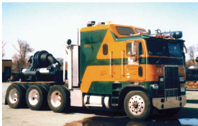
If the factory doesn't build it, do it yourself. This White Freightliner tri-axle was heavily modified. The cab was extended and an aerodyne roof was added for more living space. IT tractors numbered in the 9000 series were designated as Heavy Haul Division trucks.
