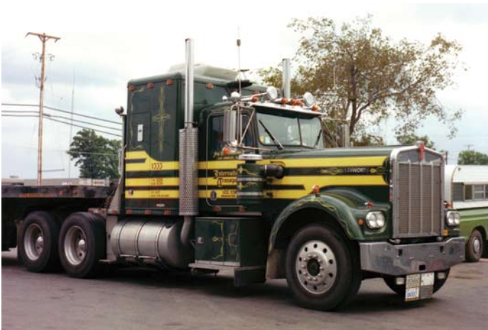
Jay Reichenbacher II from Los Angeles, CA, owned this nice Kenworth W900A extended hood tractor. The Double Eagle sleeper appears to be a 40-in unit. The tractor is also equipped with a generator, TV, roof-mounted air conditioner, and oversized fuel tanks.
