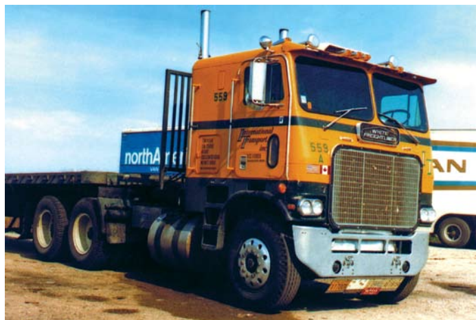
Another White Freightliner Powerliner, this one has a single bunk, 86-in cab. The Powerliner offered five different cab sizes, from 63-in day cabs up to 104-in double bunks.
